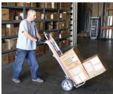
This hand truck fitted with retractable rear wheels converts into a flatbed cart.
