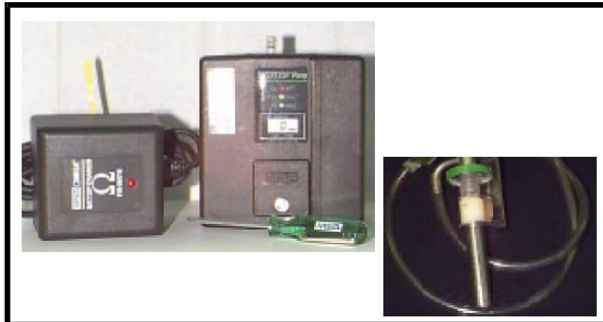
The pump has a rechargeable battery and maintains air flow at a pre-determined rate of 2.0 liters per minute. There are a number of personal sampling pumps on the market. They have similar construction and operate in a similar manner. Basically, air is drawn through the sampling train, first through the 10 mm cyclone (size selector) where nonrespirable particles are separated out as the air spins through the cyclone, then through the filter where respirable particles are deposited.
