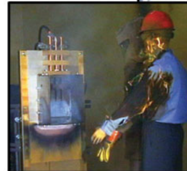
Non-FR work clothing burns after arc exposure
