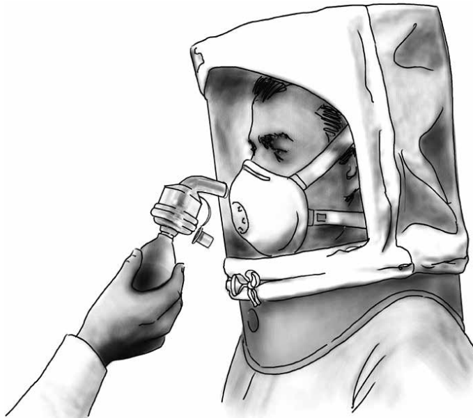
Qualitative fit testing for a disposable respirator using a special hood
