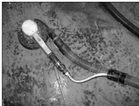
Grinder with a HEPA exhaust attachment
