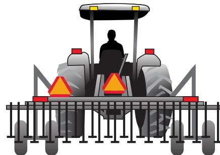
*In 34 states, SMV emblems must be displayed on the rear of any tractor and its towed attachment traveling 25 mph or slower.*
