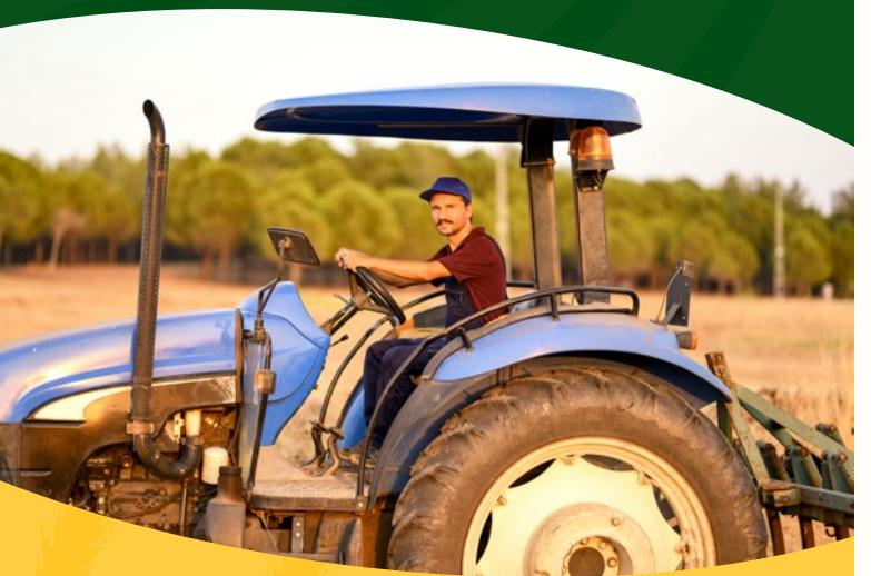
The safety of operators is increased when tractors are equipped with a rollbar or cage frame around the operator. The use of these rollover protective structures (ROPS) and a seat belt system can help reduce injuries. Many older tractors without ROPS are still in use. All tractors manufactured after October 25, 1976, must be equipped with ROPS and a seatbelt.
