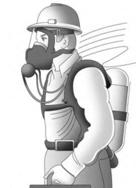
Self-Contained Breathing Apparatus (SCBA) Atmosphere-supplying, or Supplied-air respirator (SAR), which provides clean air from an uncontaminated source Needs to be fit tested APF=10,000
