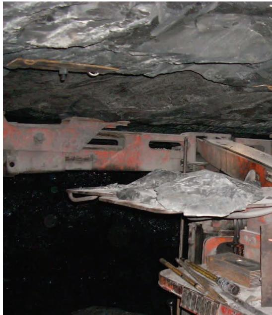
Over 95% of the 145 roof fall injuries to roof bolter operators in 2012 occurred after the ATRS system had been set.
