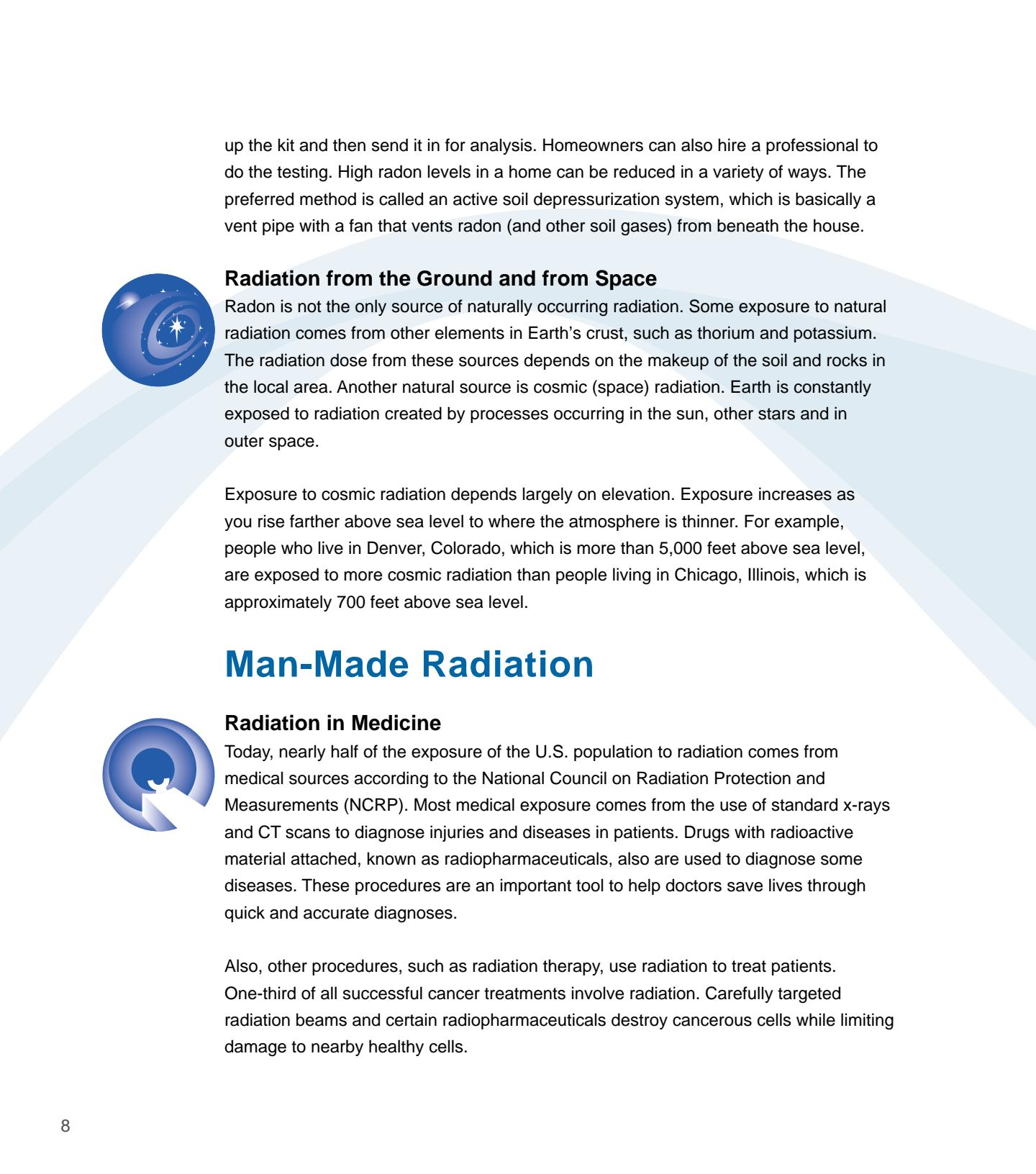
up the kit and then send it in for analysis. Homeowners can also hire a professional to do the testing. High radon levels in a home can be reduced in a variety of ways. The preferred method is called an active soil depressurization system, which is basically a vent pipe with a fan that vents radon (and other soil gases) from beneath the house.
