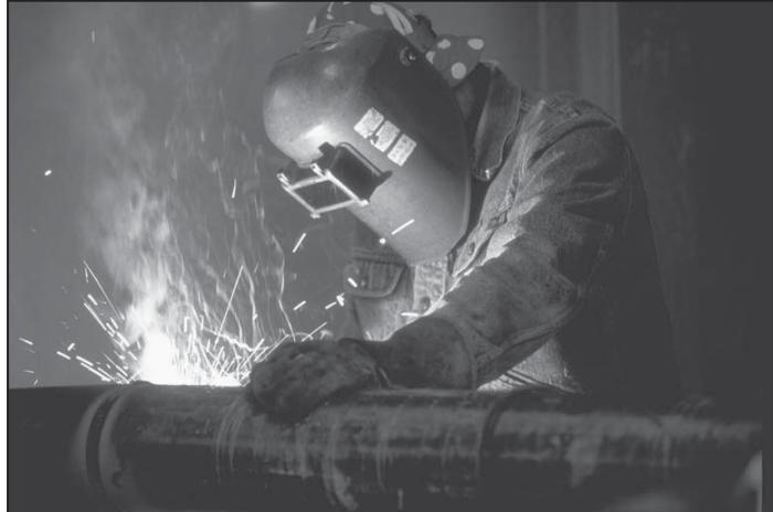
*Welding may be a source of lead exposure if lead is in the coating or in the metal being welded.*
