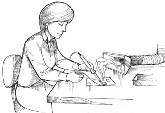
*Ventilation should draw lead fume or dust away from the work and the worker.*
