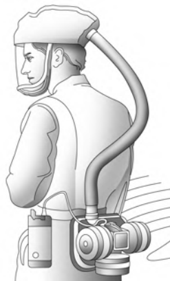
Loose-Fitting Powered Air-Purifying Respirator (PAPR) APF=25
