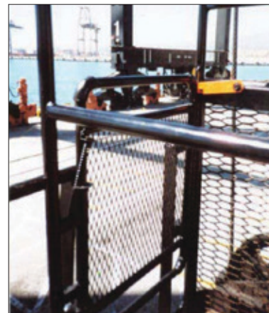
Personnel platform with locking gate
