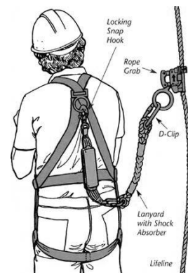
Figure 2. Components of a Personal Fall Arrest System
