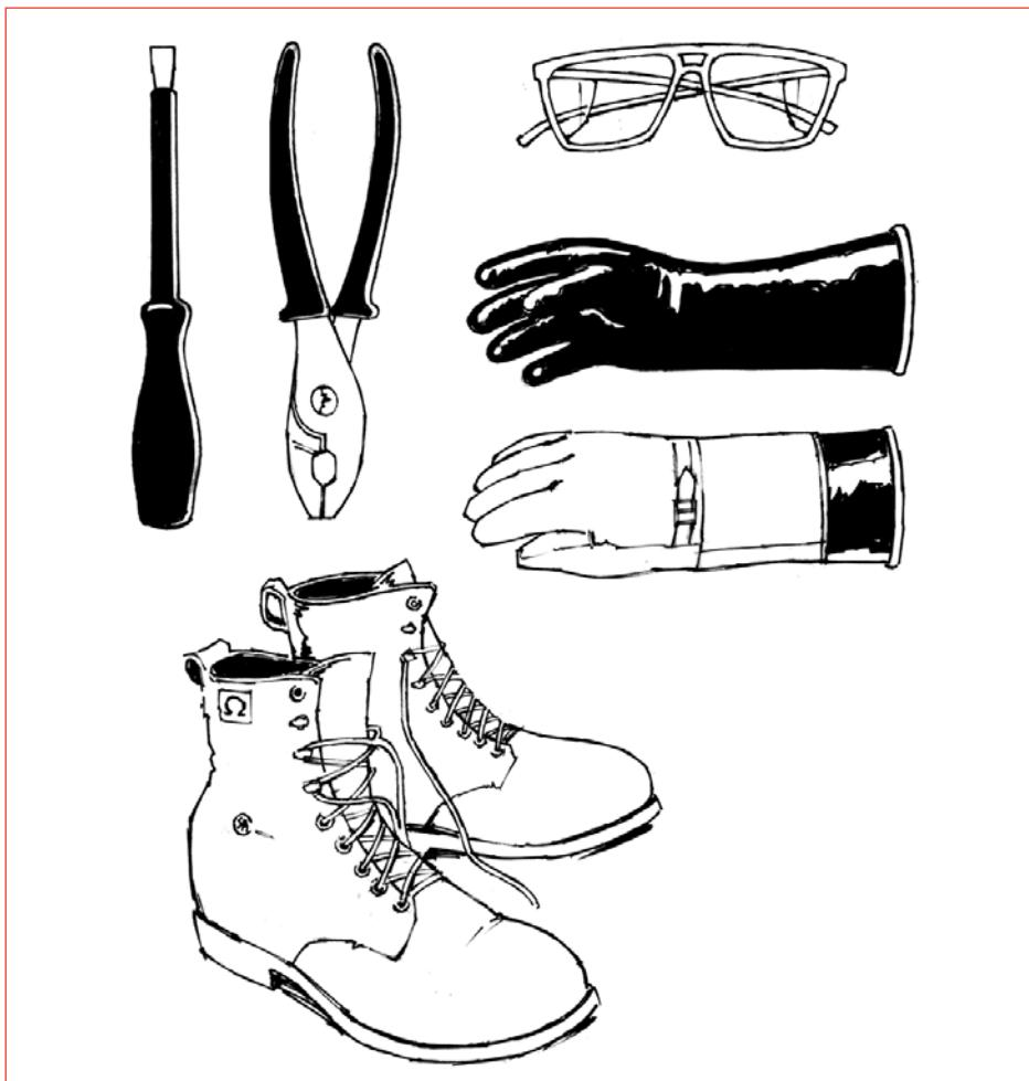
*When working on energized low-voltage equipment, workers need protective equipment, including insulated tools, safety eyewear, rubber gloves, and shock-resistant footwear.*
