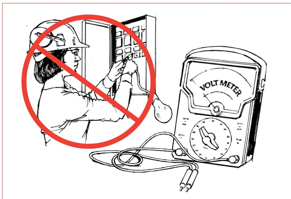
*Use approved portable meters and leads, not improvised test lamps.*
